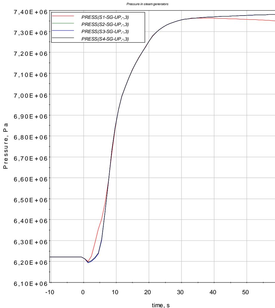
Figure 2.7 Pressure in steam generators
