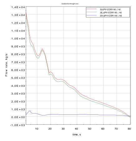
Figure 2.11 Coolant flow through core
