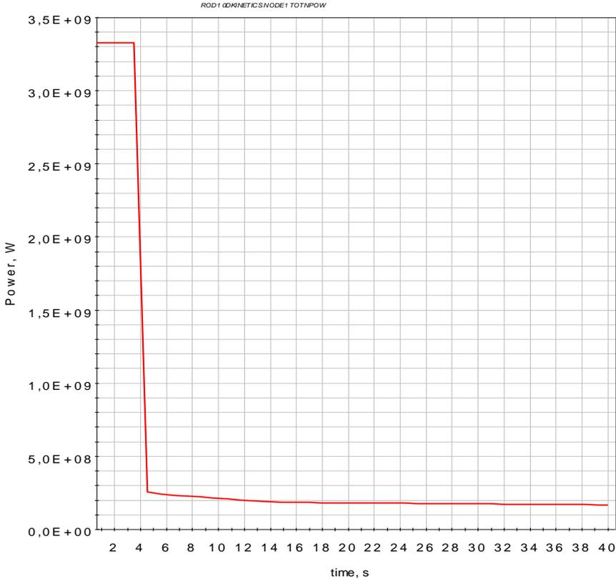
Figure 2.5 Total power of the core
