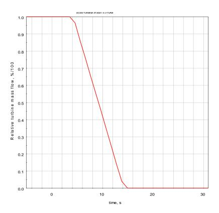
Figure 2.6 Turbine shutdown
