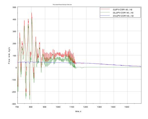
Figure 2.14 The coolant flow at the top of the core
