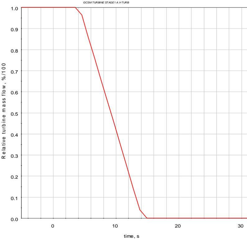
Figure 2.6 Turbine shutdown
