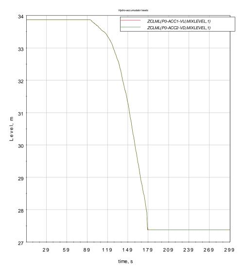
Figure 2.10 Hydro-accumulator levels (absolute height values)
