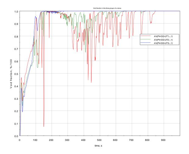
Figure 2.13 Void fraction in the three groups of u-tubes
