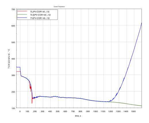
Figure 2.15 The coolant temperature at the top of the core
