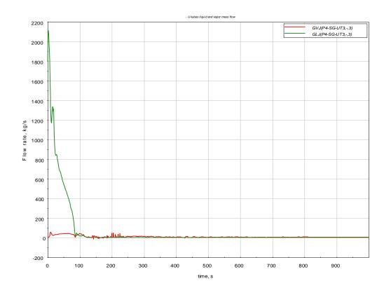
Figure 2.12 U-tubes liquid (green) and vapor (red) mass flow
