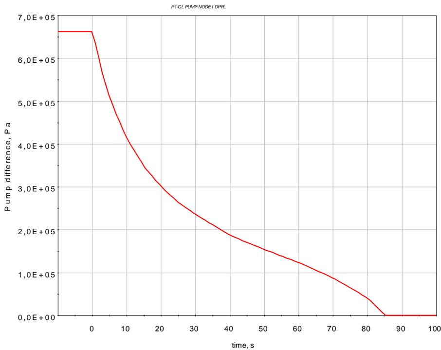
Figure 2.4 Main circulation pump head
