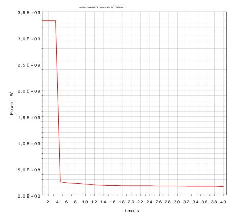
Figure 2.5 Total power of the core
