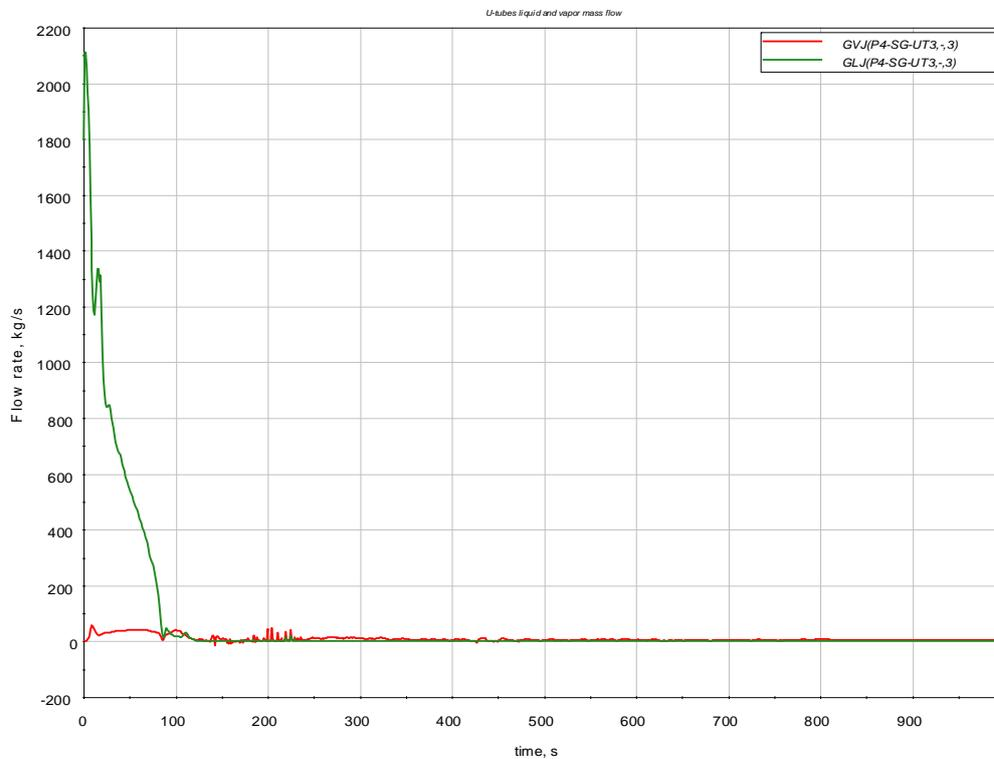
Figure 2.12 U-tubes liquid (green) and vapor (red) mass flow
