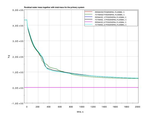
Figure 2.1 Residual water mass together with total mass for the primary system (red, green  $-1^{st}$  case, blue, black  $-2^{nd}$  case, purple, azure  $-3^{rd}$  case)
