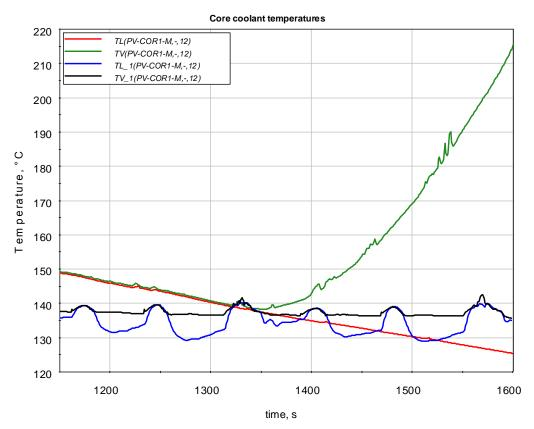
Figure 3.11 Core coolant temperatures (2<sup>nd</sup> case) green curve: BDBA vapor temperature; black curve: DBA vapor temperature
