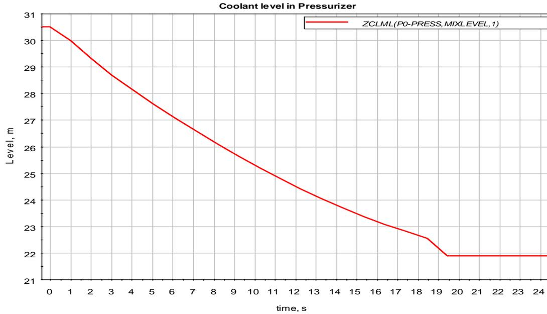
**Figure 2.6 Coolant level in Pressurizer**
