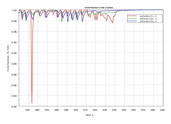
Figure 2.17 Void fraction in the three groups of u-tubes
