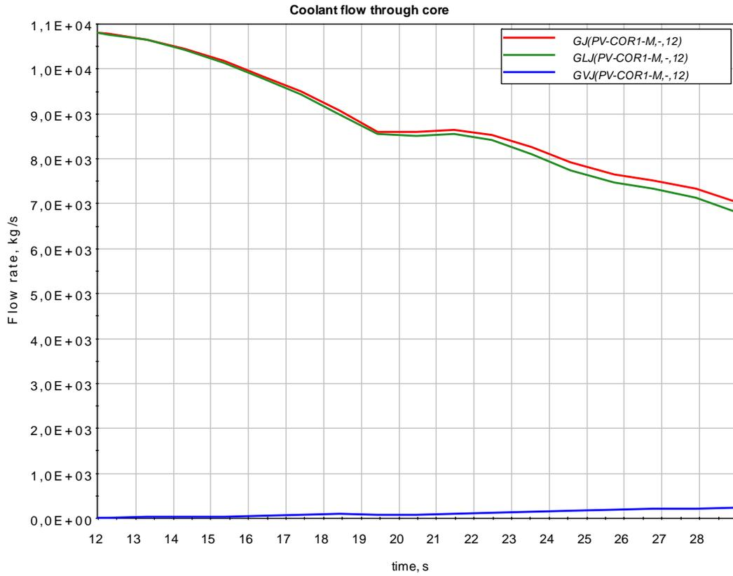
Figure 2.15 Coolant flow through core
