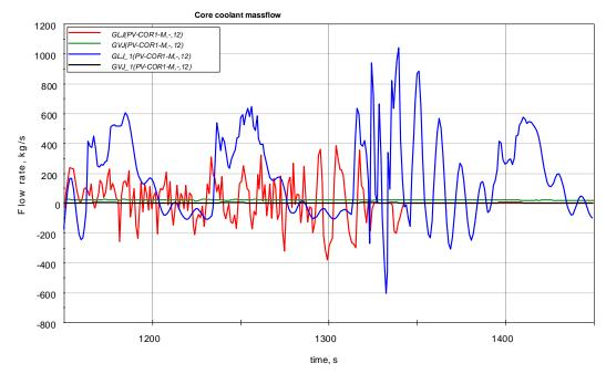
Figure 3.9 Core coolant massflow (2<sup>nd</sup> case) red/green curves: BDBA; blue/black curves: DBA
