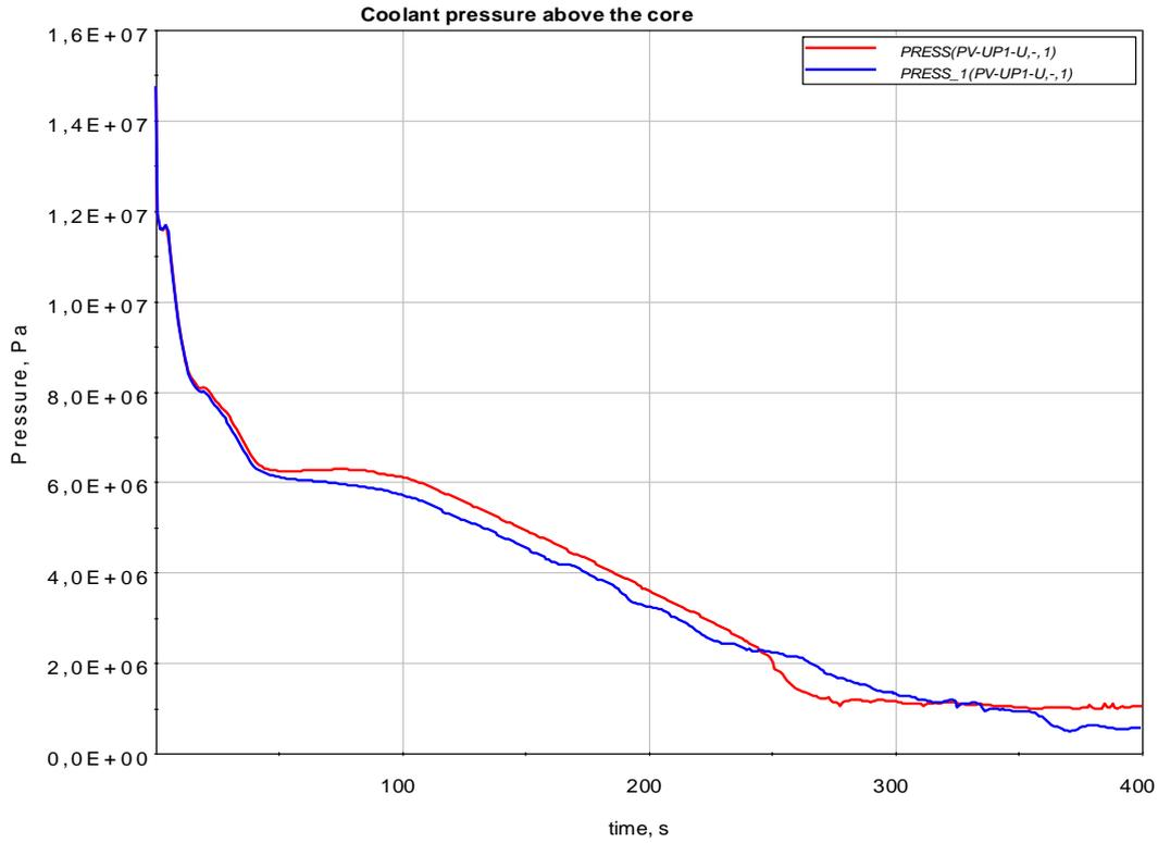
**Figure 3.1** Coolant pressure above the core (PV-UP1-U, 1<sup>st</sup> case)
