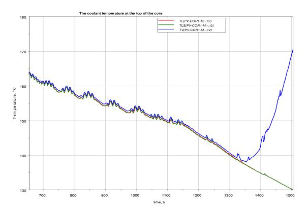
Figure 2.19The coolant temperature at the top of the core
