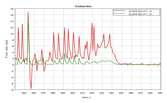
Figure 2.16 U-tubes liquid (green) and vapor (red) mass flow
