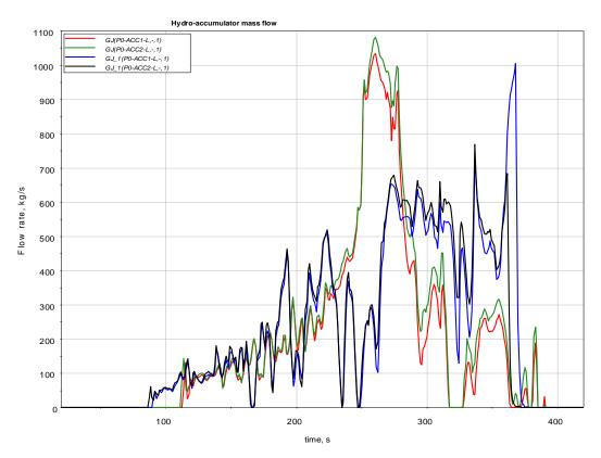
Figure 3.2 Flowrate from hydro-accumulators (1<sup>st</sup> case) red/green curves: BDBA; blue/black curves: DBA
