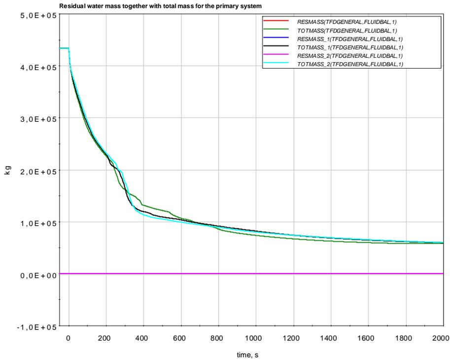
**Figure 2.1** Residual water mass together with total mass for the primary system (red, green – 1<sup>st</sup> case, blue, black – 2<sup>nd</sup> case, purple, azure – 3<sup>rd</sup> case)
