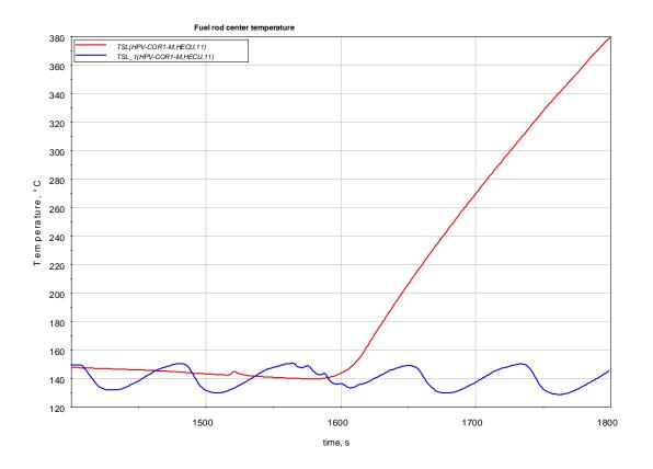
Fuel rod center temperature (2<sup>nd</sup> case) Figure 3.12 red curve: BDBA; blue curve: DBA
