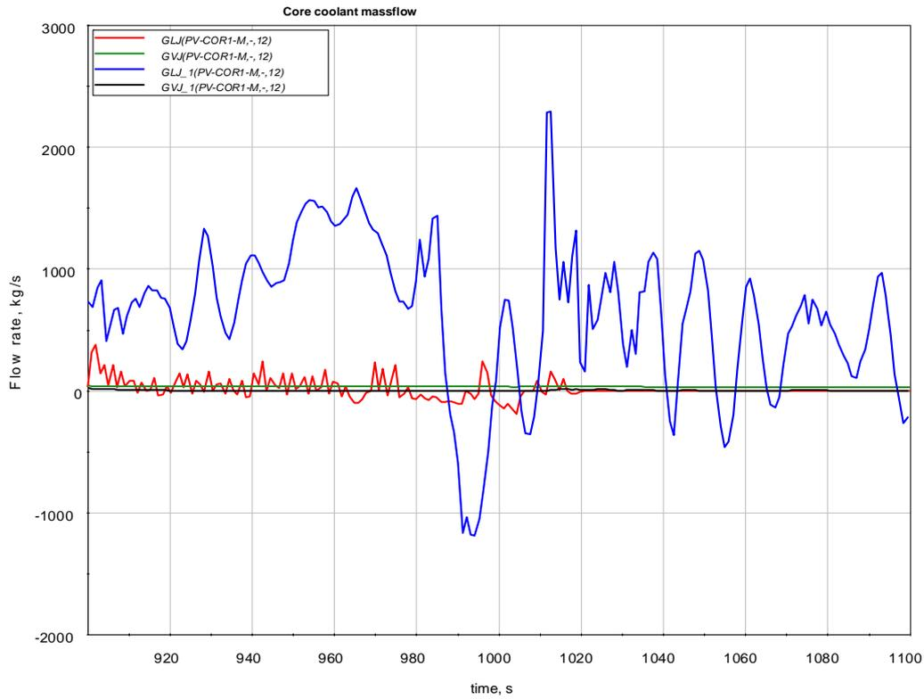
**Figure 3.5 Core coolant mass flow (1<sup>st</sup> case) red/green curves: BDBA; blue/black curves: DBA**
