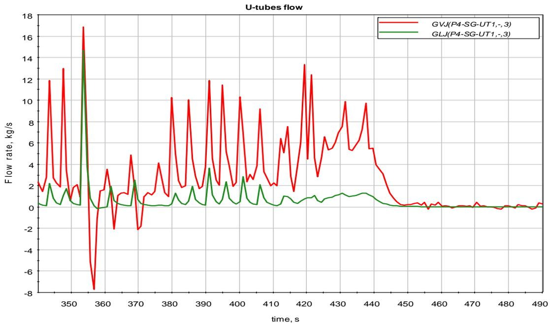
Figure 2.16 U-tubes liquid (green) and vapor (red) mass flow
