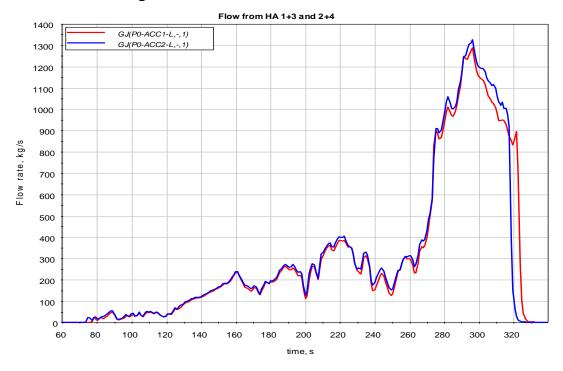
Figure 2.13 Hydro-accumulator mass flow
