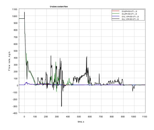
Figure 3.3 U-tubes coolant flow (1<sup>st</sup> case) red curve: BDBA, vapor; green curve: BDBA, liquid; blue curve: DBA, vapor; black curves: DBA, liquid
