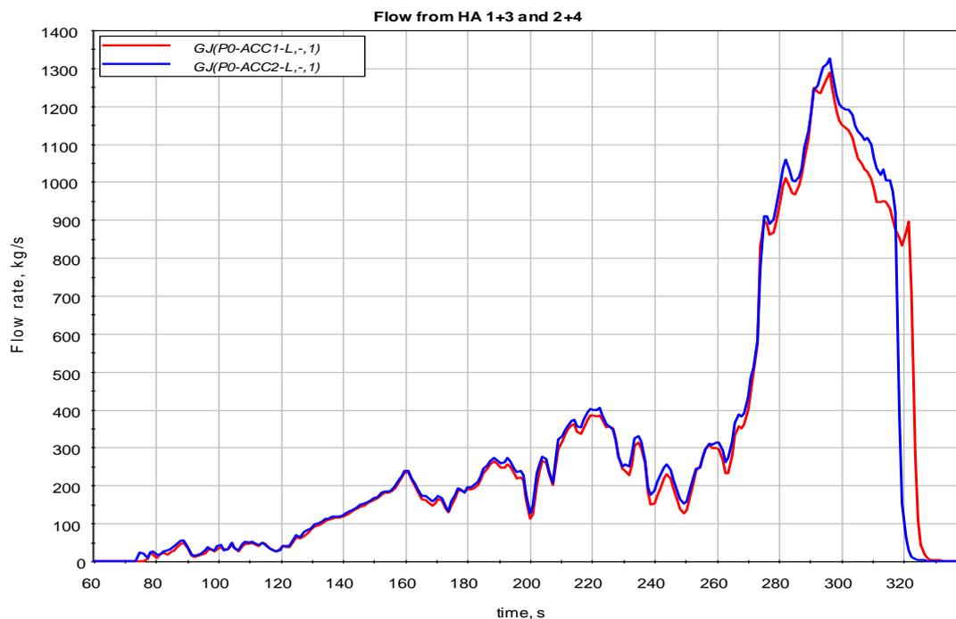
**Figure 2.13** Hydro-accumulator mass flow
