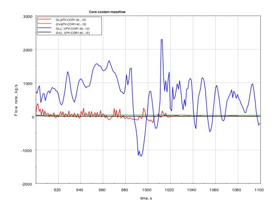
Figure 3.5 Core coolant mass flow (1<sup>st</sup> case)red/green curves: BDBA; blue/black curves: DBA
