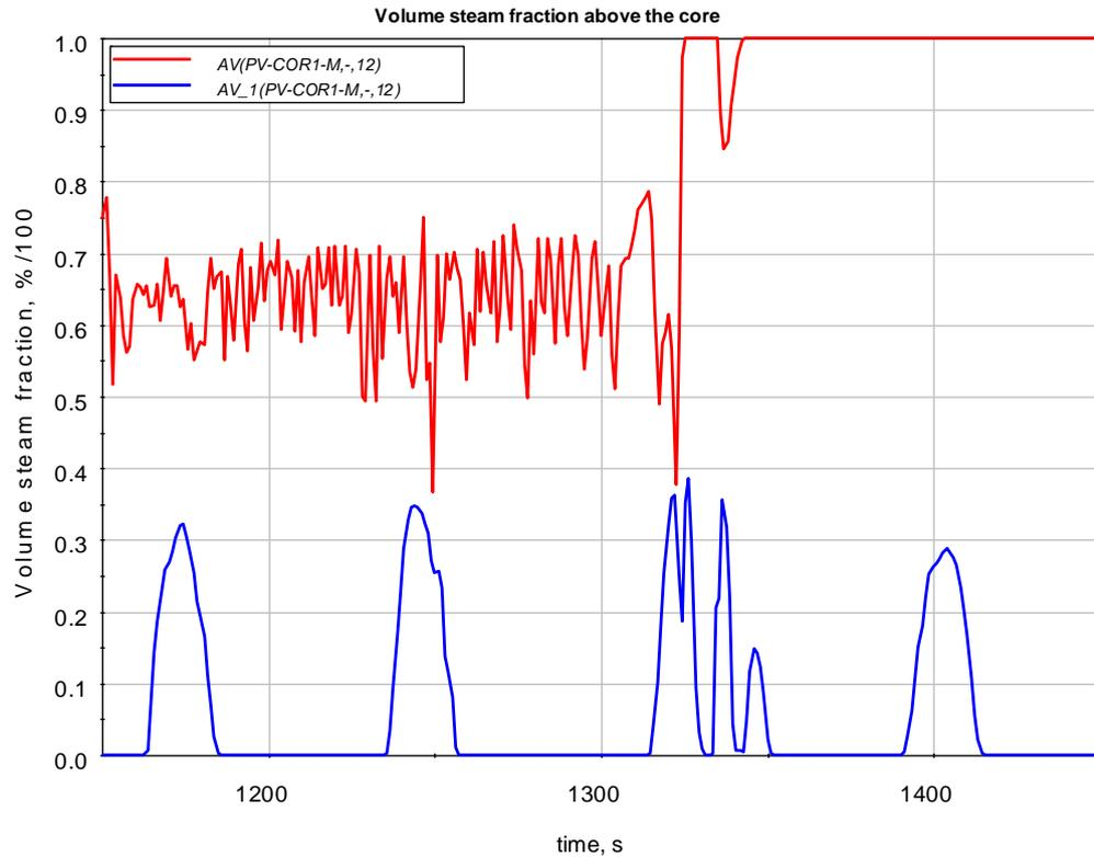
**Figure 3.10** Volume steam fraction above the core (2<sup>nd</sup> case)
