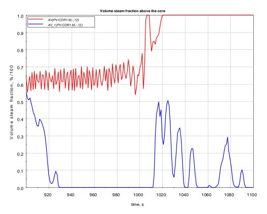
Figure 3.6 Volume steam fraction above the core (1<sup>st</sup> case) red curves: BDBA; blue curves: DBA
