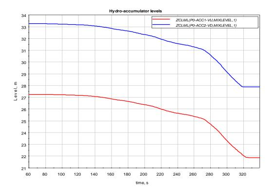
Figure 2.14 Hydro-accumulator levels (absolute height values)
