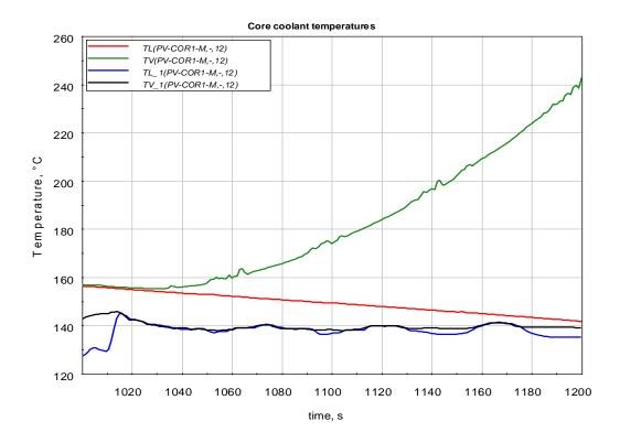
**Figure 3.7 Core coolant temperatures (1<sup>st</sup> case)** green curve: BDBA vapor temperature; black curve: DBA vapor temperature
