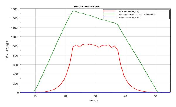
Figure 2.12 BRU-A and BRU-K operation red curve: BRU-K mass flow rate; blue curve: BRU-A mass flow rate; green curve: critical discharge rate of BRU-K (= maximum possible mass flow through the valve)
