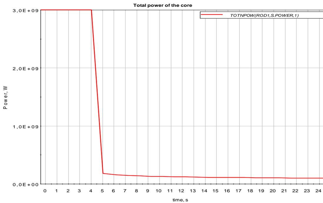
**Figure 2.9 Total power of the core**
