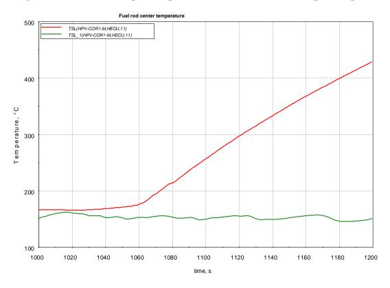
Figure 3.8 Fuel rod center temperature (1<sup>st</sup> case) red curve: BDBA; blue curve: DBA
