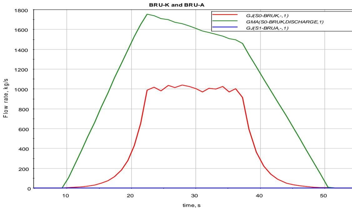
**Figure 2.12 BRU-A and BRU-K operation**
