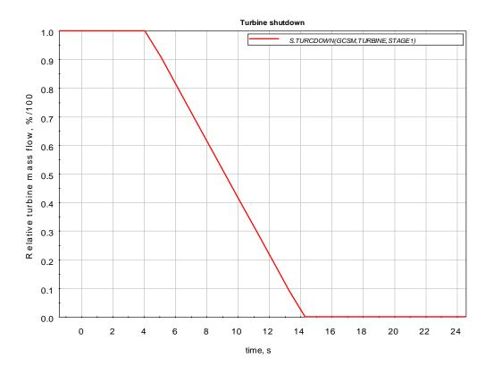
Figure 2.10 Turbine shutdown
