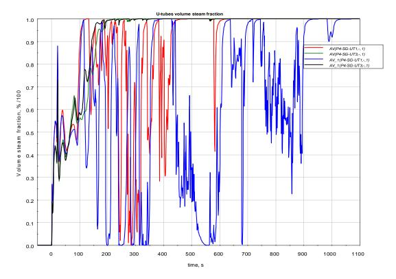
Figure 3.4 U-tubes volume steam fraction (1<sup>st</sup> case) red/green curves: BDBA; blue/black curves: DBA
