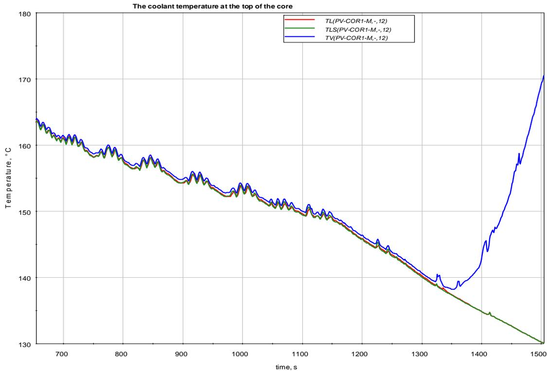
**Figure 2.19** The coolant temperature at the top of the core
