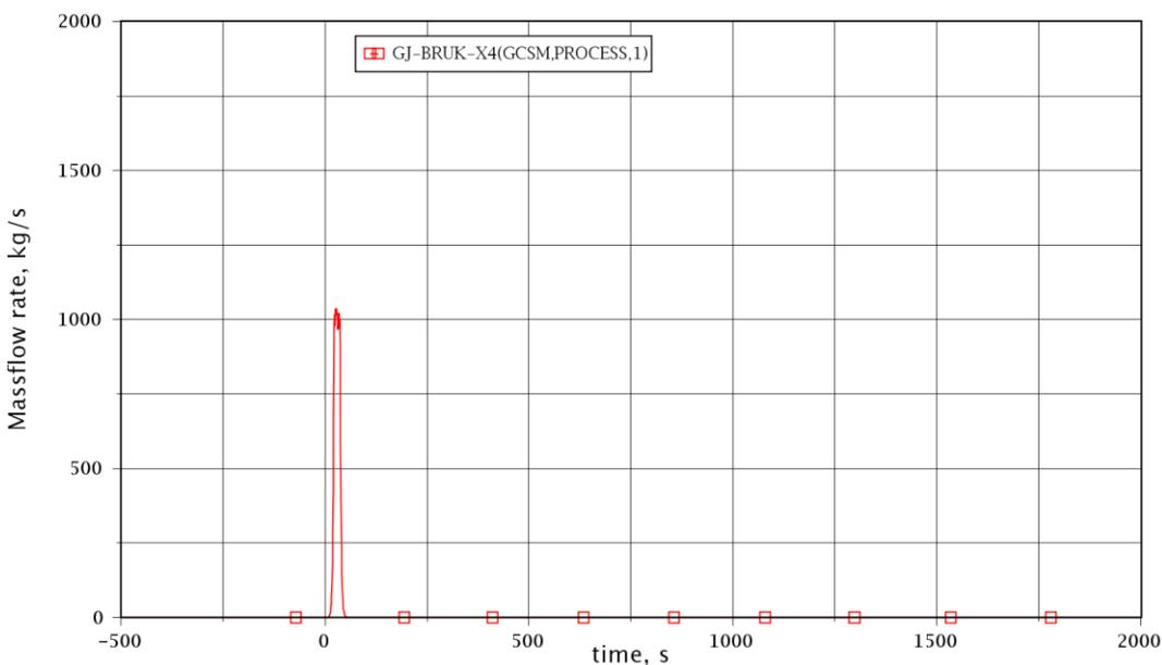
**Figure 2.4 BRU-K mass flow rate (2<sup>nd</sup> case)**
