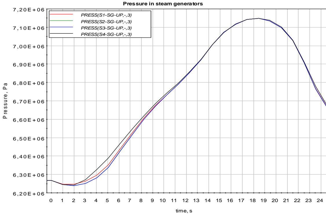
**Figure 2.11 Pressure in steam generators**
