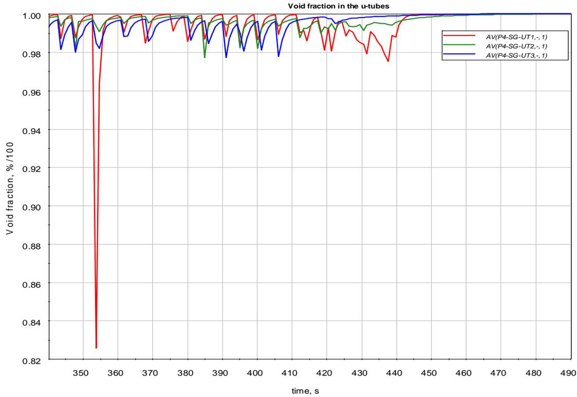
**Figure 2.17** Void fraction in the three groups of u-tubes
