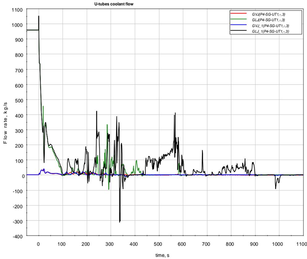
**Figure 3.3 U-tubes coolant flow (1<sup>st</sup> case)**
