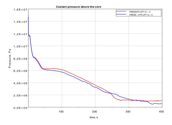
Figure 3.1Coolant pressure above the core (PV-UP1-U, 1st case)<br/>blue curve: DBA; red curve: BDBA
