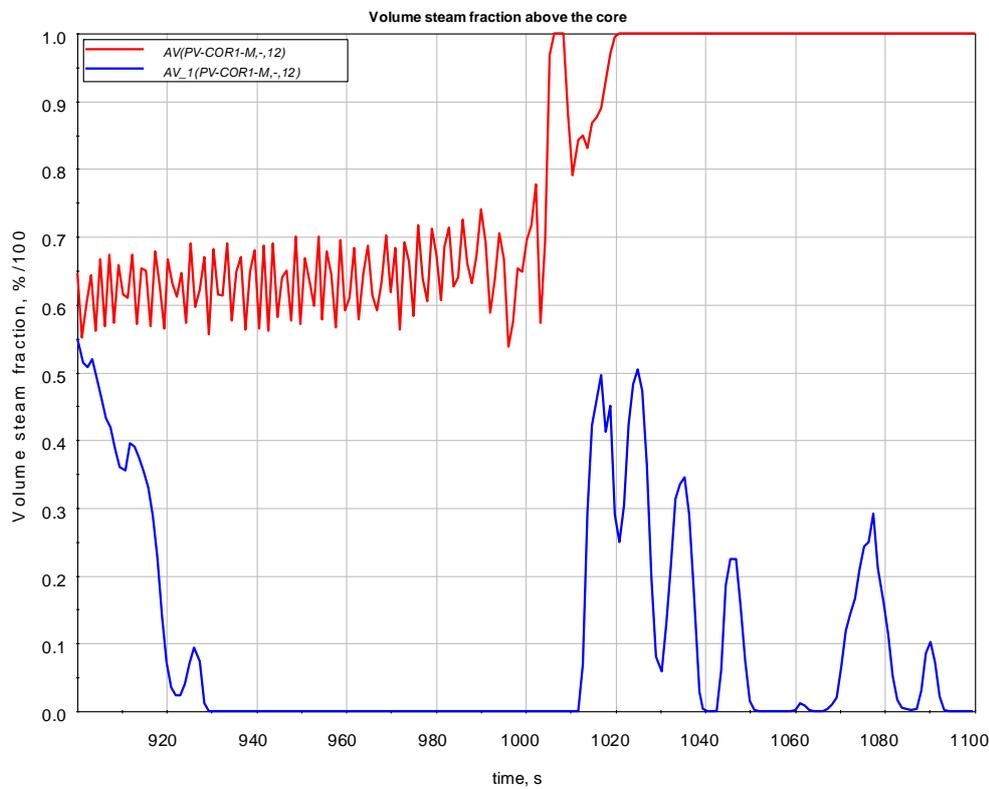
**Figure 3.6 Volume steam fraction above the core (1<sup>st</sup> case) red curves: BDBA; blue curves: DBA**
