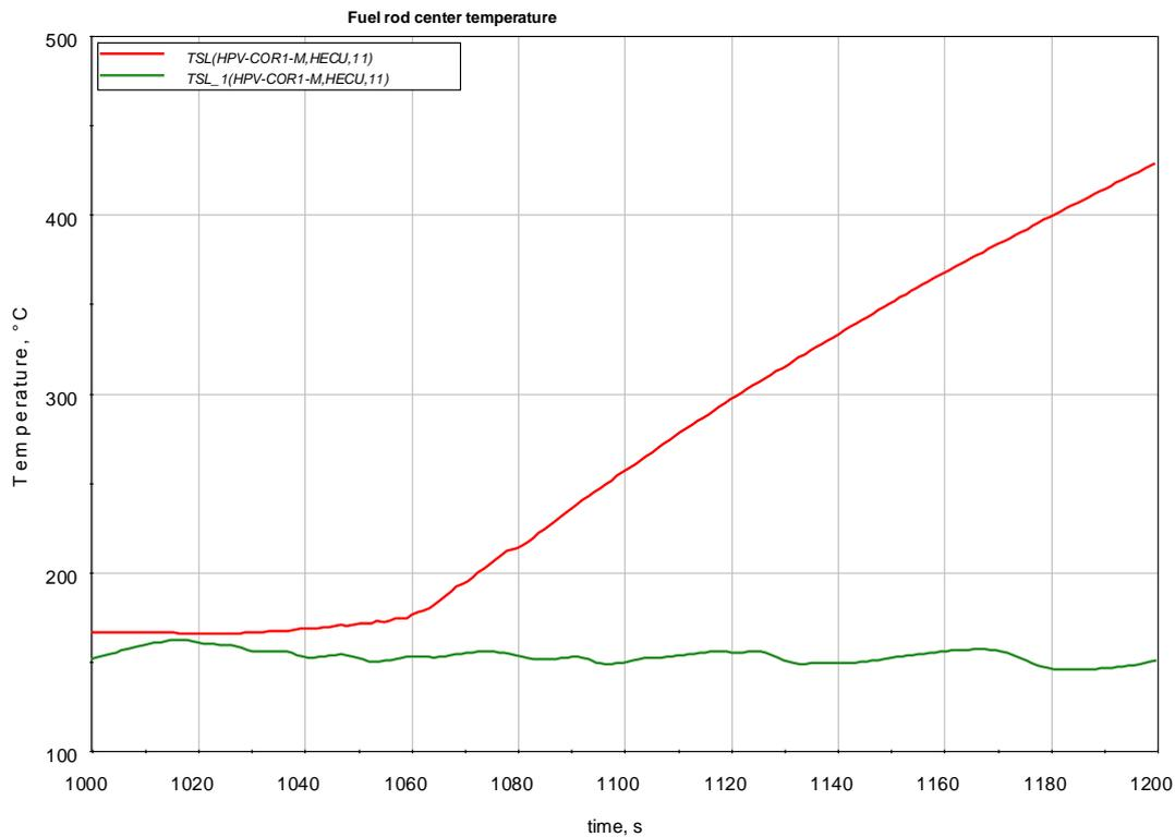
**Figure 3.8 Fuel rod center temperature (1<sup>st</sup> case)**
