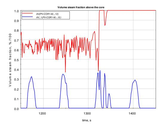
Figure 3.10 Volume steam fraction above the core (2<sup>nd</sup> case) red curves: BDBA; blue curves: DBA
